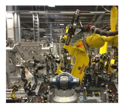
The 13<sup>th</sup> R-Dist Parameter gives the possibility to measure a Point "after" the last Axis mounted anywhere at the Tool.
